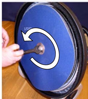
4. Insert and tighten the centre screw. NOTE! Tighten counter clockwise!
