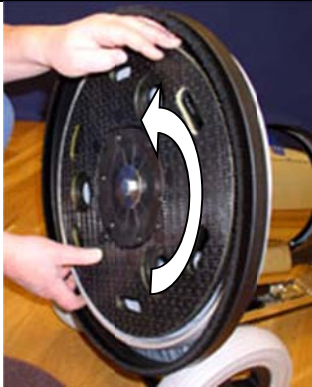
3. Mount the Pad Drive. NOTE! Mount counterclockwise!
