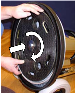
1. Mount the Pad Drive and loosen the center screw. NOTE! Loosen clockwise!
