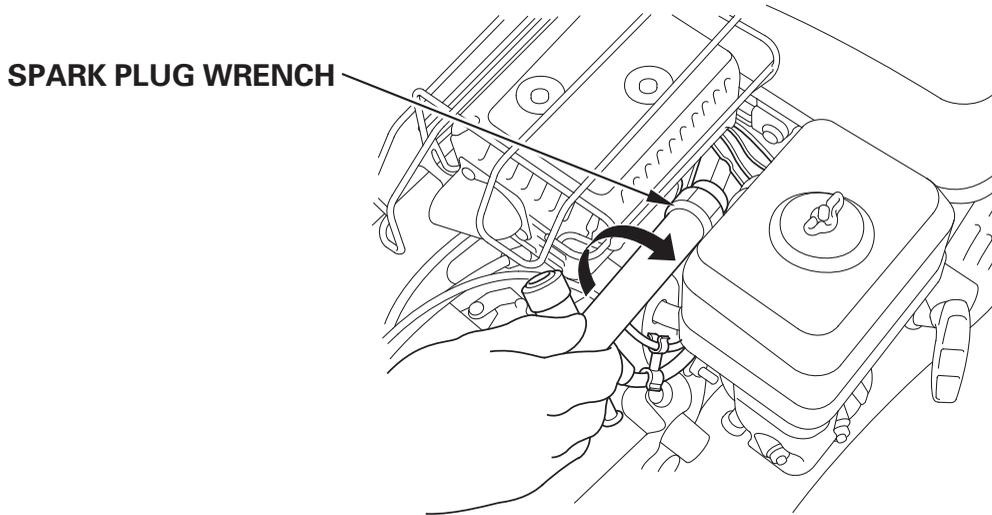
5. After the spark plug is seated, tighten with a spark plug wrench to compress the washer.
