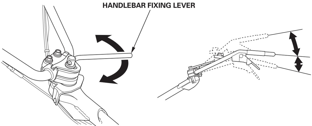
If the handlebar angle adjustment is needed, loosen the handlebar fixing lever, move the handlebar to a required position and tighten the lever.
