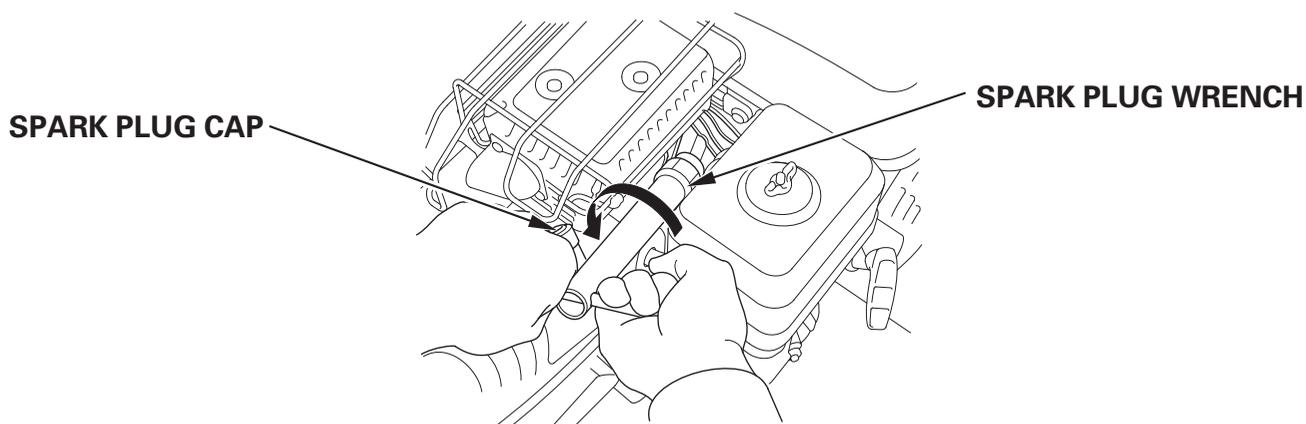
2. Visually inspect the spark plug. Discard it if the insulator is cracked or chipped. Clean the spark plug with a wire brush if it is to be reused.
