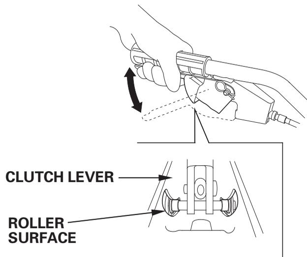
To clean the clutch lever roller, disassemble the clutch lever (see page 25 ).
