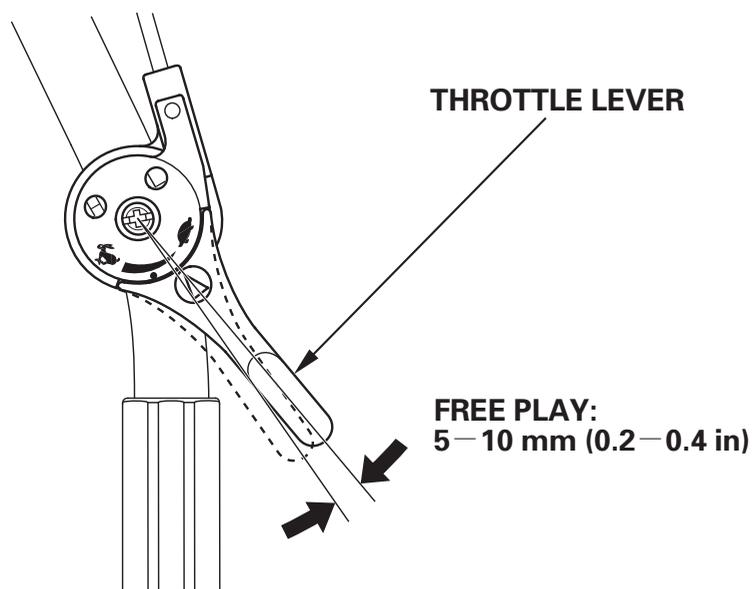
If the free play is incorrect, loosen the lock nut and turn the adjusting nut in or out as required.
