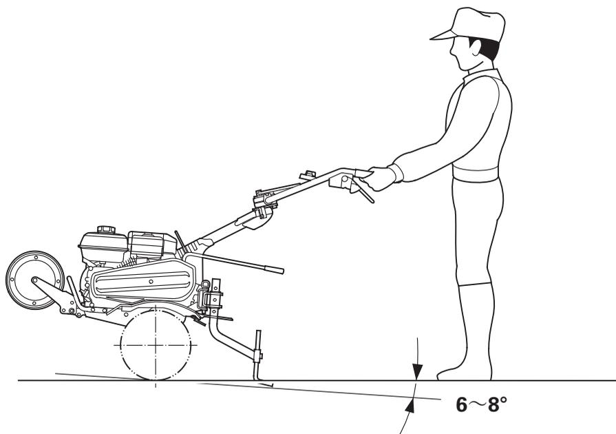
To get the maximum advantage from the tiller, try to hold the machine at the angle shown while you are tilling the ground:
