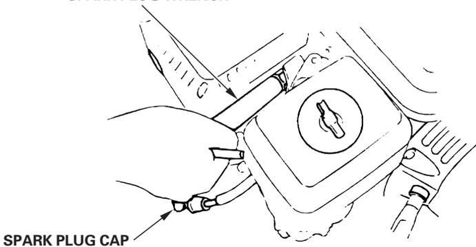
3. Inspect the spark plug. Replace it if the electrodes are worn, or if the insulator is cracked or chipped.
