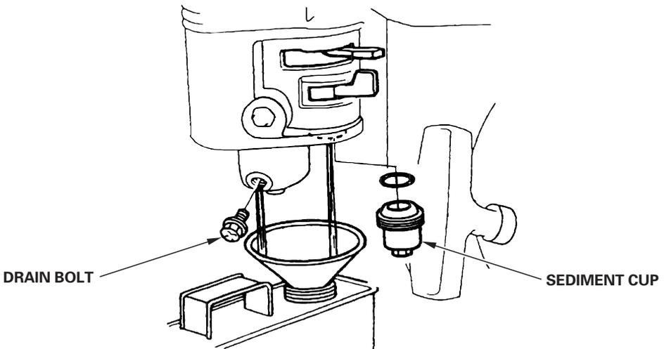
3. After all the fuel has drained into the container, reinstall the drain bolt and sediment cup. Tighten them securely.
