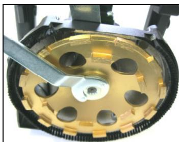
Use the face spanner to unscrew the driving nut.
